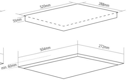
If installed without a gap in between, cut-out width = [no. of hobs - 1] x 288mm + 268mm
