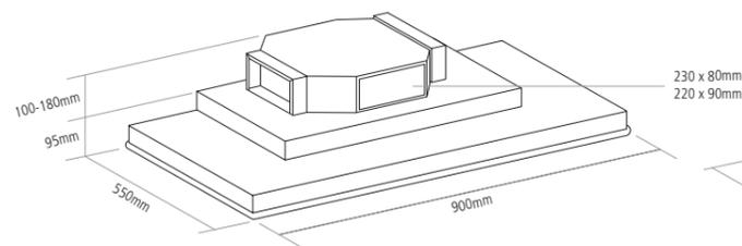
For installation into the ceiling a niche of 865mm by 515mm is required, with a minimum height of 200mm
