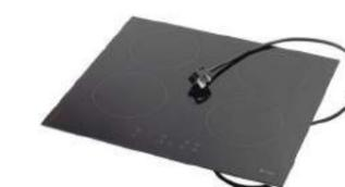
PLEASE NOTE: The C840i induction hob achieves a 13A connection by restricting the maximum load to 3kW, this is done by cleverly limiting the combined zones to a maximum power level sum of 12. For example if you had boiling water on power level 6 on one zone you could cook rice on power level 4 and gently warm food on level 2 on a third zone.
