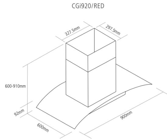
Note: Suitable to be installed in a standard room height of 2.3m
