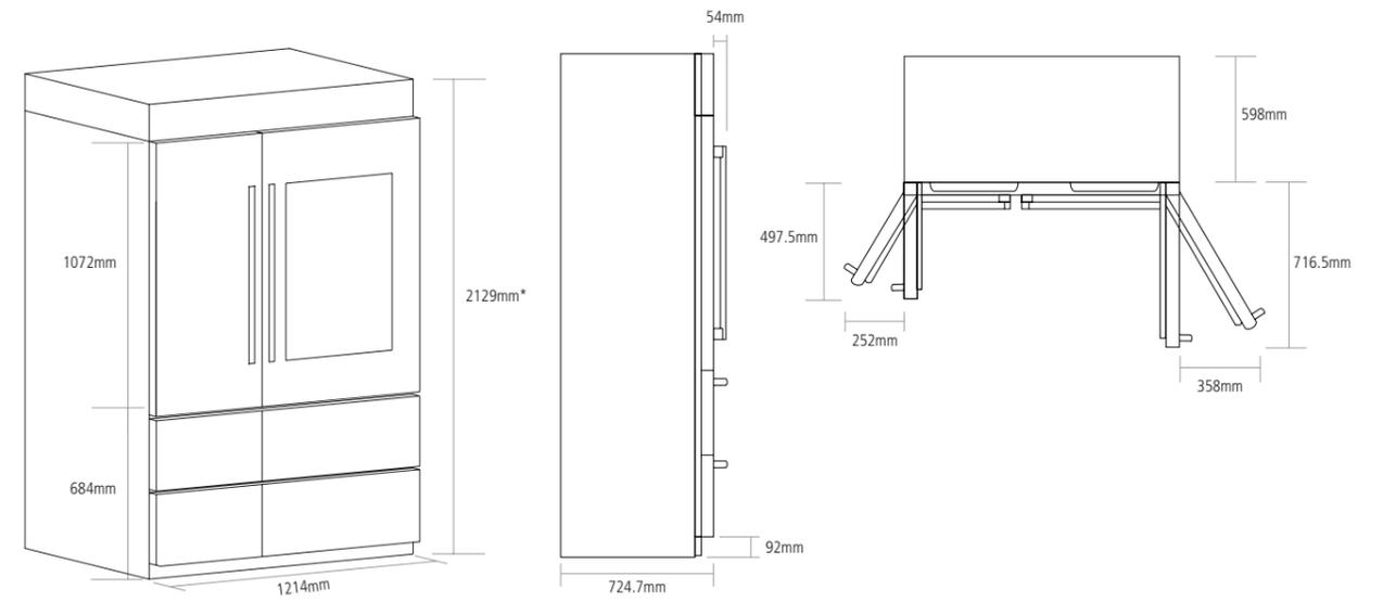
\*Height of Product when feet are not extended, 2136mm when feet are extended.
