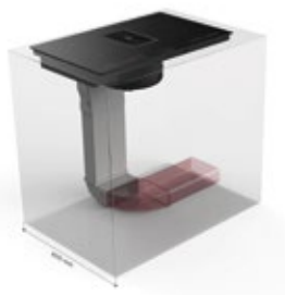
Lateral ducting version installation
